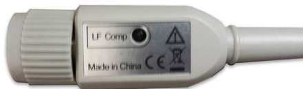
Figure 2. Low-frequency compensation adjustment (for N2840A/41A/42A/43A/53A)
